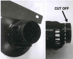
2 Remove remains of nose using a flat screw driver or pliers
