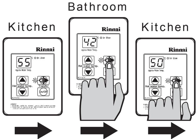
Depending on the weather conditions and the length of the pipe between the heater and the tap in use, there may be a variation between the temperature displayed at the controller and the temperature at the tap.
