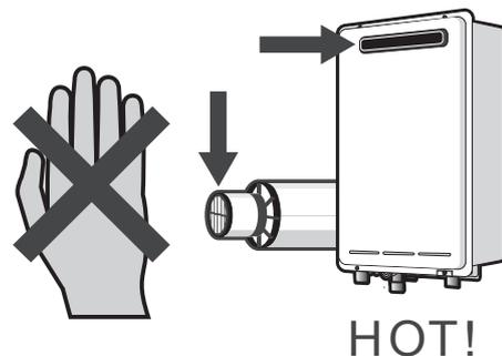
On cold days steam may be discharged from the flue outlet. This is normal, do not be alarmed. It does not indicate a fault.
